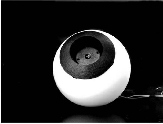
Fig. 6. Assembled eye-ball (camera cables shown in background)
