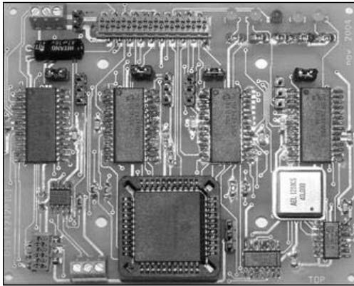
Fig. 15. The embedded real-time controller. The board has dimensions of  $69 \times 85$  <sup>2</sup> to be integrated with the eye
