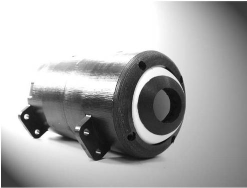
Fig. 11. MAC-EYE assembled (without camera)
