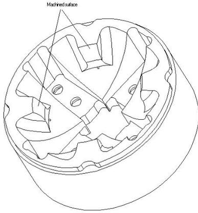
Fig. 10. Detail of the flange supporting the eye-ball.
