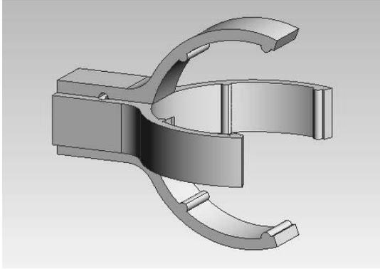
Fig. 7. CAD model of the eye-ball support.
