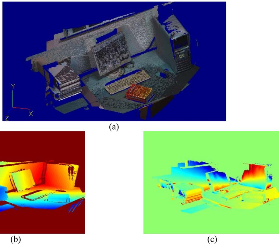
**Figure 4:** Results obtained with the VR simulator. (a) The 3D model of an indoor scene, acquired by the laser scanner. (b-c) Horizontal and vertical ground truth disparity maps, for a given fixation point.
