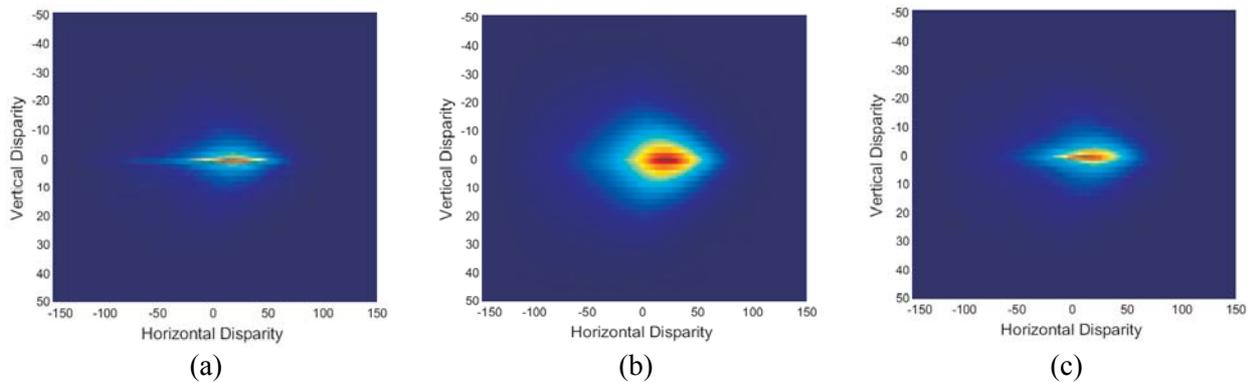
**Figure 3:** Comparative analysis of the probability distribution of horizontal and vertical disparities for the three different stereo-head systems considered: (a) a classical Tilt/Pan system; (b) a system following Listing's Law; (c) a system following *L2*.
