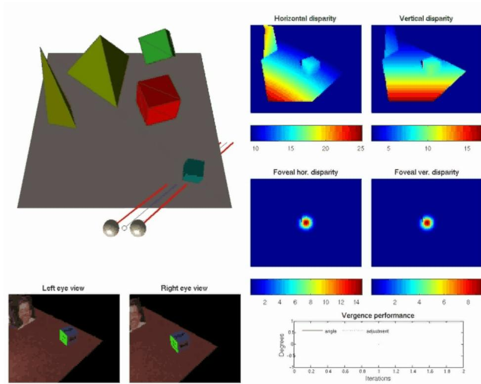
**Figure 6:** Top left panel: realistic scene lay-outs with stereo set-up (eyes) and fixation point in 3D. Bottom left two panels: views obtained after ray-tracing for the two eyes. Top right two panels: horizontal and vertical disparities corresponding to the fixation point. Middle right two panels: distribution of vertical and horizontal disparities when performing vergence. Bottom right panel: vergence control as a function of time.
