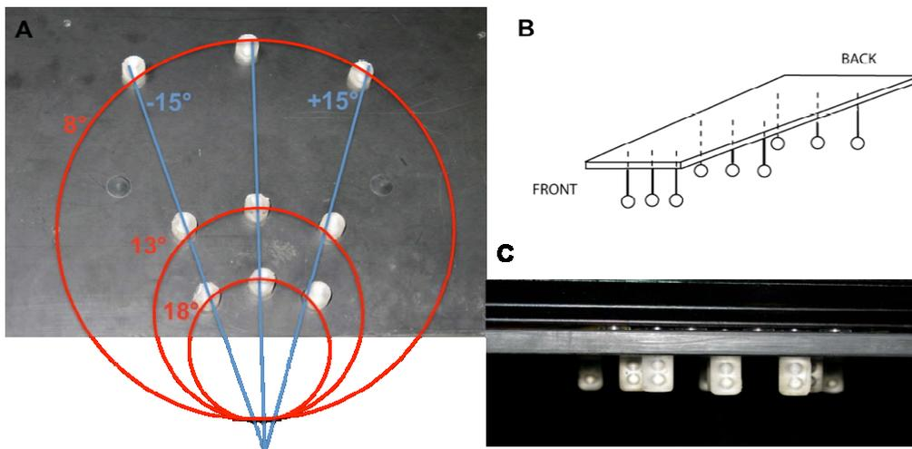
**Figure 24:** The fixation-in-depth/reach-in-depth device. Each of the 9 targets contains a green/red bicolor LED use to instruct the monkey, and an embedded microswitch used to check target pressing. A) Bottom view of the device superimposed with isoversion (blue) and isovergence (red) lines. B) General prospect of the device. C) Frontal view of the device (as seen from the monkey side).
