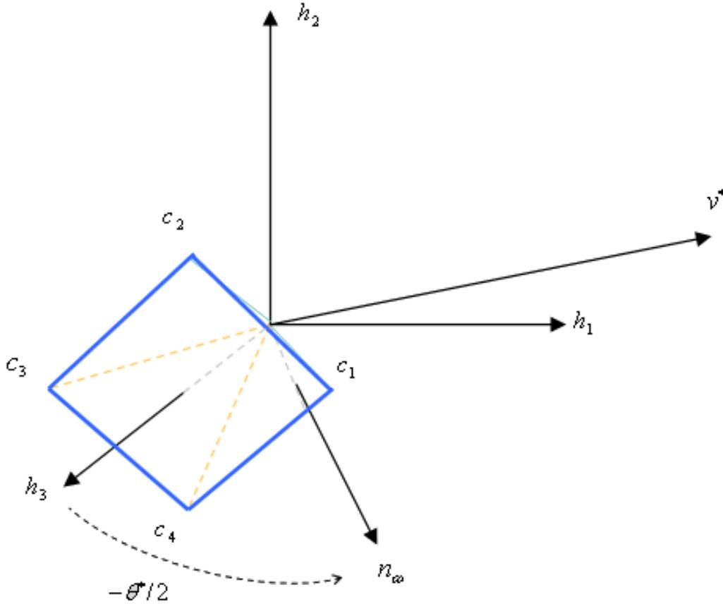
Figure 9: Geometry of the oculomotor plant after a rotation  $(\mathbf{v}^*, -\theta^*)$ :  $\mathbf{n}_\omega^R$  vector  $\perp$  to the Half-Angle Plane, the vectors  $\mathbf{r}_i$  and vector  $\mathbf{e}_3$  are rotated back in primary position.
