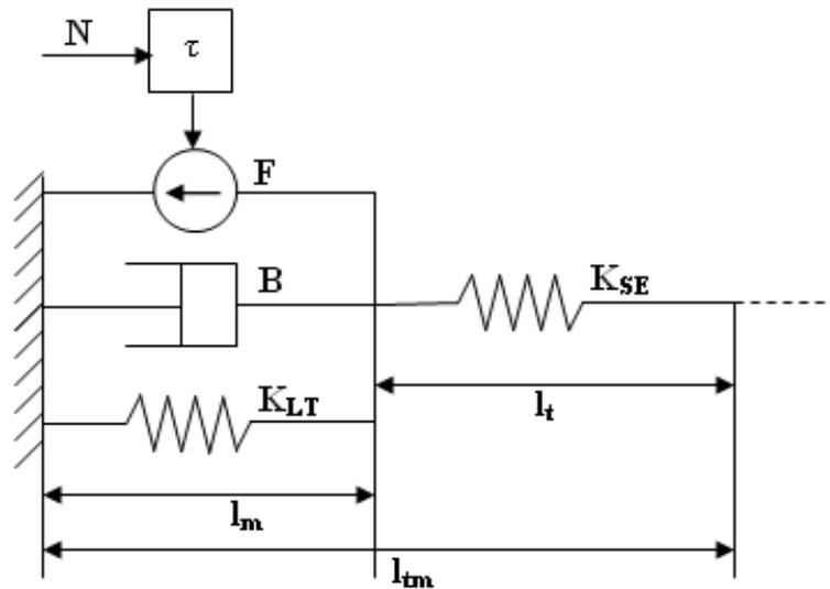
Figure 7: Linearized muscle model:  $F$  active state tension generator,  $B$  viscosity element,  $K_{LT}$  tendon elastic element,  $K_{SE}$  muscle elastic element.
