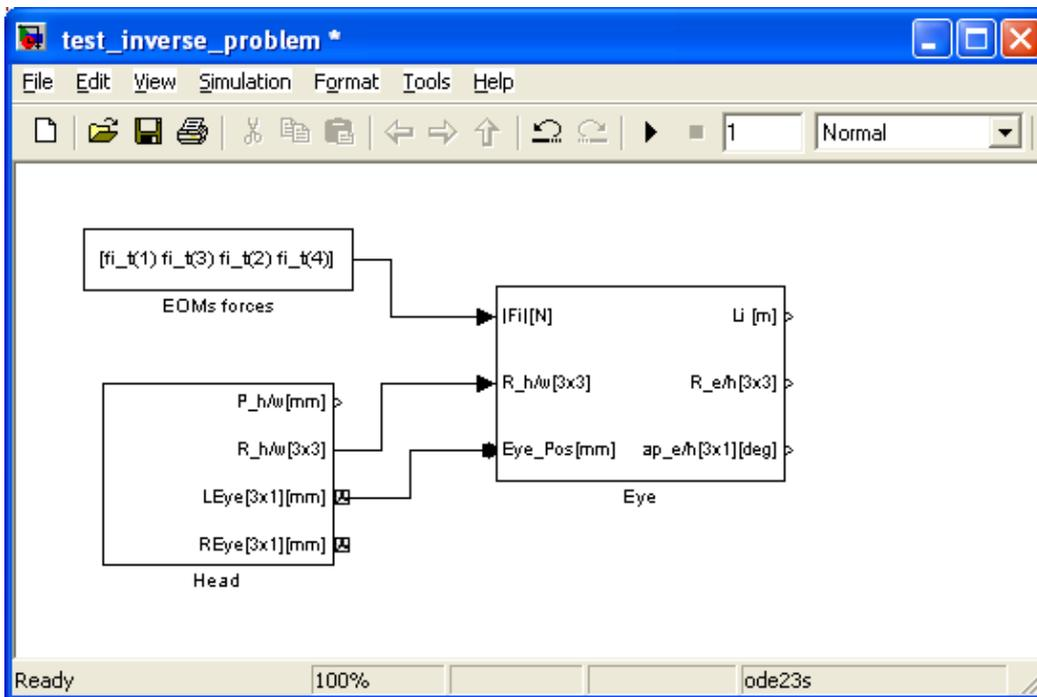
Figure 12: Simulink model of the oculomotor plant, composed of the head, the eyeball and the four muscle forces (constats).
