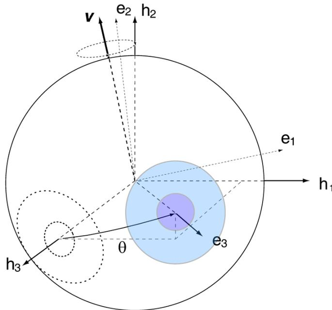
Figure 3: Geometry of Listing compatible rotations. The finite rotation axis  $\mathbf{v}$  is always orthogonal to  $\mathbf{h}_3$ .  $\theta$  is the amount of rotation about  $\mathbf{v}$
