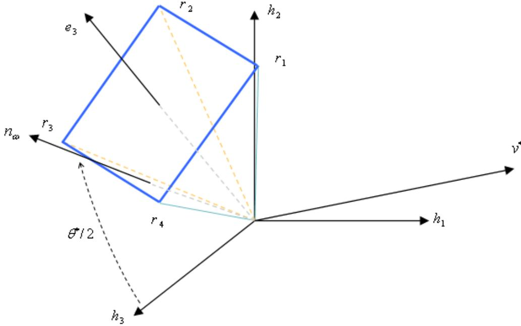
Figure 8: Geometry of the oculomotor plant after a rotation  $(\mathbf{v}^*, \theta^*)$ :  $\mathbf{n}_\omega$  vector  $\perp$  to the Half-Angle Plane,  $\mathbf{r}_i$  new position of the four insertion points.
