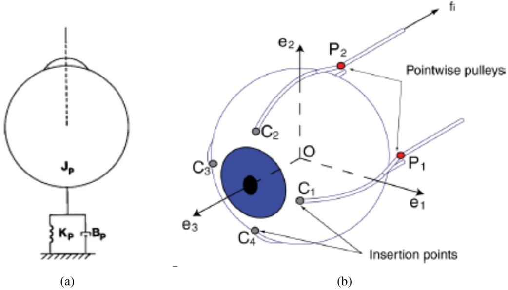
Figure 5: Mechanical and geometrical model of the oculomotor plant. (a) Sketch with the mechanical parameters of the human eye:  $J_p$  moment of inertia,  $B_p$  orbit viscosity and  $K_p$  orbit elasticity. (b) Sketch of the eye at the primary position, according to the assumptions made on the placement of IPs, PPs, and routing of the EOMs. Each EOM generates a pulling force  $f_i$ .
