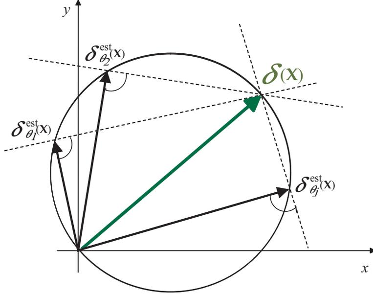
Figure 1: Recovery of the 2D disparity vector. By construction, the end points of all the (correct) estimates  $\delta_{\theta}^{est}$  of the disparity component with respect to the orientation  $\theta$  are located on a circle through the origin. The true full disparity is the longest vector whose end point lies on the circle.
