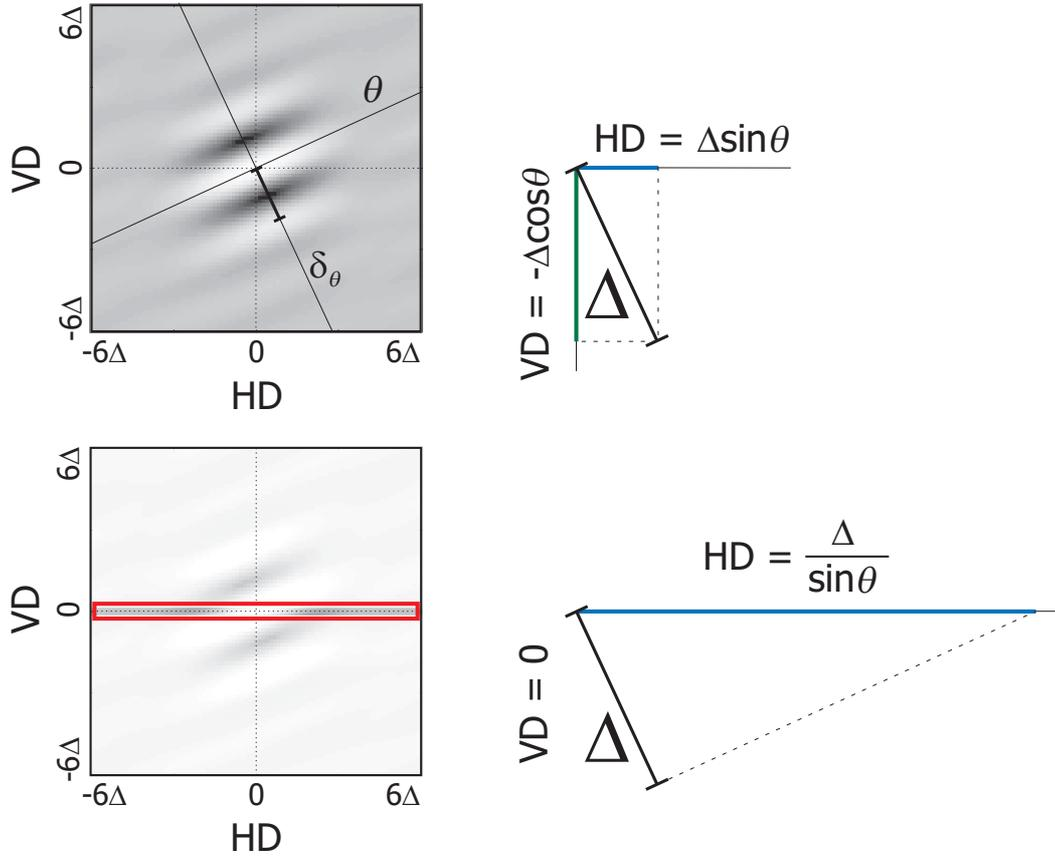
Figure 6: Each complex cell is, by construction, tuned to an oriented disparity  $\delta_\theta$ , *i.e.*, each cell is jointly tuned to horizontal (HD) and vertical (VD) disparities. (Top): For each oriented disparity, its contribution to the HD and VD is calculated by projections on the horizontal and vertical lines. (Bottom): By assuming  $VD=0$ , the orientation of the RF is used as a degree of freedom to extend the sensitivity range of the cell to horizontal disparity stimuli (HD).
