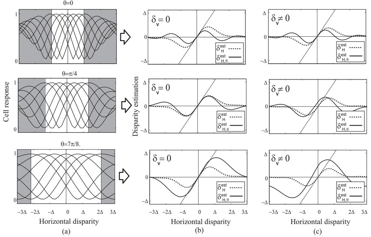
Figure 7: (a) Disparity tuning curves of complex cells at different orientations. (b) Estimated horizontal disparity using single orientation channels in presence of horizontal disparity only ( $\delta_V = 0$ ). (c) Estimated horizontal disparity using single orientation channels in presence of a fixed amount of vertical disparity ( $\delta_V \neq 0$ ). Dashed line plots refer to the horizontal disparity estimates obtained by combining all the orientation channels.
