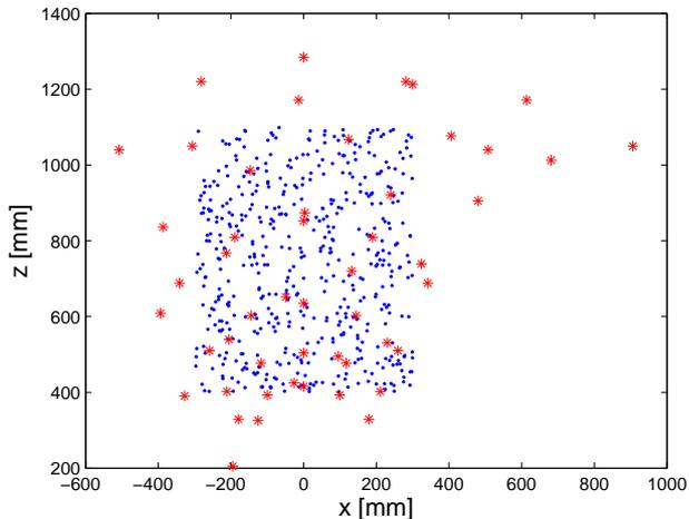
Fig. 6. Radial basis functions distributed according to a mixed criterion (25 oculomotor + 25 arm motor, red stars), visualized over a typical Cartesian training set (blue dots).
